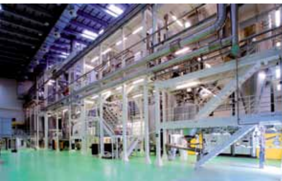
A pre-refiner sends cocoa mass toward a series of five-roll refiners for initial processing.
