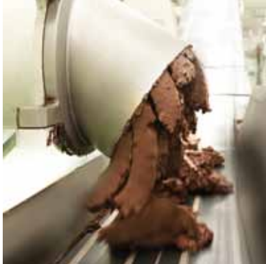
A pre-refiner sends cocoa mass toward a series of five-roll refiners for initial processing.
