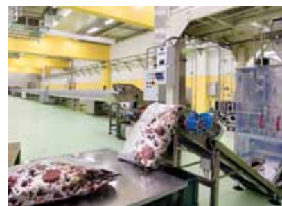
An automated bagger handles chocolate chips as they come off the line.
