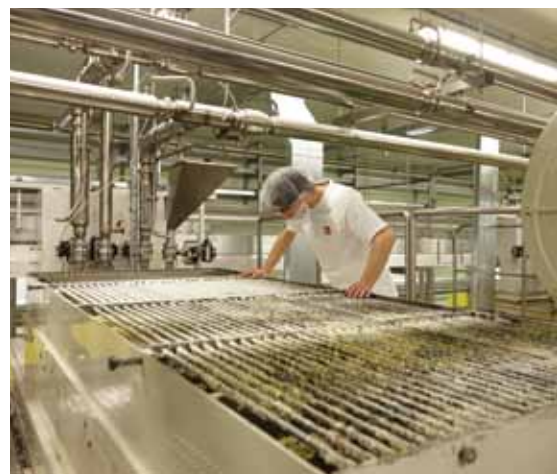
A production worker inspects conching of white chocolate. The company has seven conches that typically process chocolate from 8 to 12 hours.
