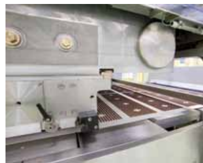
A 1.5-meter wide depositor turns out a high volume and broad range of chocolate chip couvertures.
