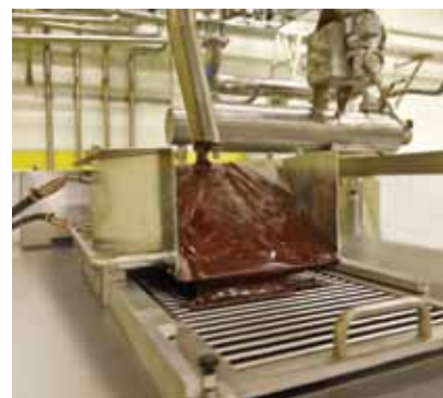
Chocolate is deposited onto a chocolate chips production line.
