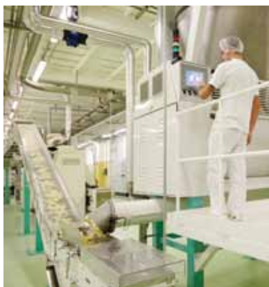
A production worker inspects conching of white chocolate. The company has seven conches that typically process chocolate from 8 to 12 hours.
